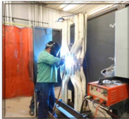
Dale Bowman stud welding.
